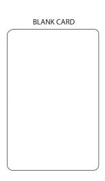
Half-sized YMC Panels: Full-color images and graphics can be printed anywhere on the card. The maximum color print area is 34 millimeters in height when the card is in portrait position. (See red lines in Exhibit A.)
