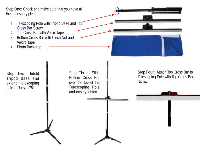
Step Five: Remove the Velcro Tape from the Top Cross bar. Attach Backdrop to Top Cross Bar by hooking the backdrop grommet on the nipple on one side. Line up the Velcro, and pulling tightly across to the other side, snap the grommet over the nipple on the other side so as to carefully line up both sides of the Velcro.
