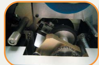
Patented integrated flipper and magnetic stripe encoder
