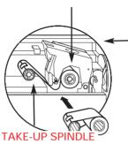
3. Load ribbon onto the supply spindle (under print head carriage) and empty core (with tape attached) onto the take-up spindle flange side in. Make sure the ribbon comes off of the top of the supply spindle and feeds to the top of the take-up spindle.
