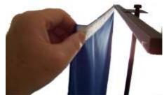
Step Six: Repeat the same procedure for the bottom edge of the Backdrop. Do not tighten bottom bar completely until the Backdrop is lined up on the top and bottom – Then pull the Bottom Cross Bar down to take out the slack and wrinkles from the Backdrop-Well Done!
