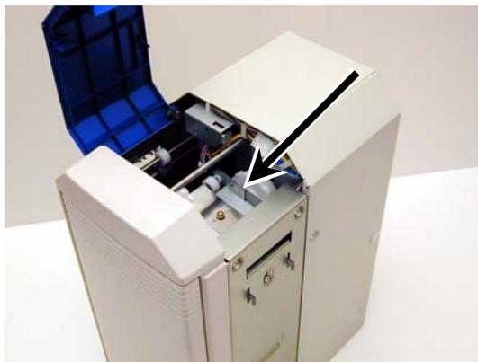
5. Clean each of the flip/turn rollers (white plastic and rubber) using an alcohol swab.
