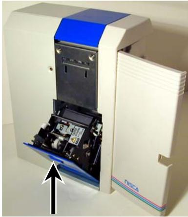
4. Open the front access cover and slide the laminate ribbon rollers onto the two white drive hubs. The notches on the take-up spool and supply roll should face inward.
