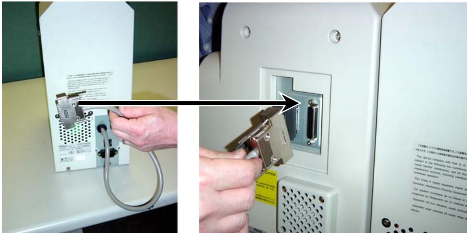
5. Attach the card stacker into the mounting slots.
