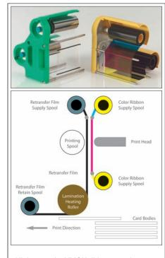
High-capacity YMCK ribbon together with the separate re-transfer film provides 1000 color prints.
