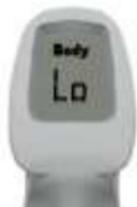
When using the ThermoFlash LX-26 the message Lo can show on the screen.
