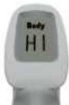
When using the ThermoFlash LX-26 the message HI can show on the screen.
