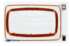
to communicate with an external antenna. The chip is a piece of semi-conducting material (usually composed of silicon) on which an integrated circuit is embedded. It has only one function: to provide the prox card reader with the card's identification number and/or site facility code number so it can be verified on a remote computer.
